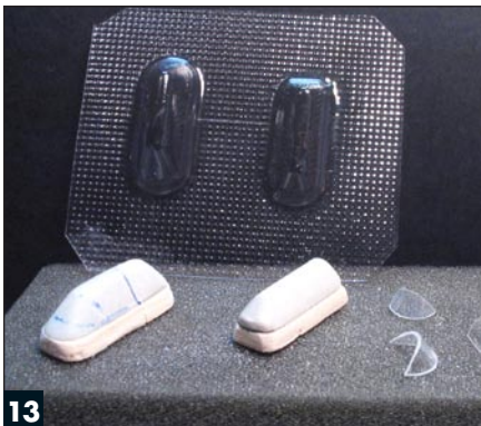
13 Using epoxy-putty molds, Rato vacuum-formed canopy parts. The left mold is for the windscreen and canopy, the right for the rear section.
