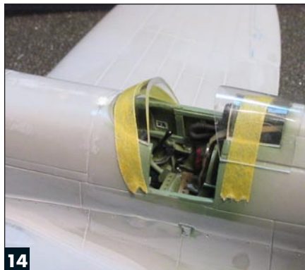
14 Rato dry-fits the vacuum-formed canopy parts, refining the shape carefully to ensure a tight fit with the fuselage.
